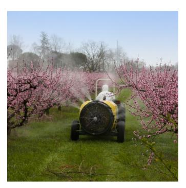
High static pressure to push the fertilizer through the nozzles, and resistance to sudden changes in the fan speed are the most important characteristics to keep in mind when you have to choose the right fan for your agricultural sprayer.
